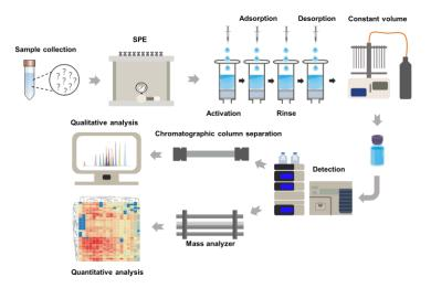
In conclusion, the developed SPE-UPLC-MS/MS method effectively overcomes the matrix challenges of refinery wastewater, providing high sensitivity, accuracy, and robustness for monitoring trace-level PFAS, thereby fulfilling a critical need for environmental monitoring in the petroleum industry.
